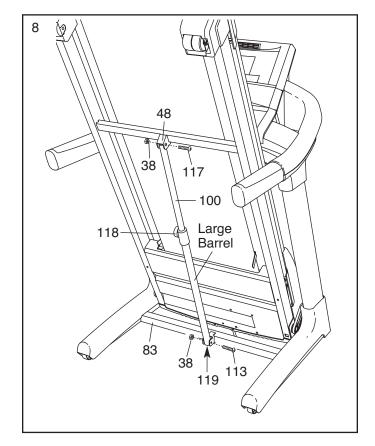
With the help of a second person, raise the front of the treadmill and insert the crossbar on the Base (83) into the cutout in the cardboard stand as shown. Have the second person hold the treadmill to prevent it from moving forward or backward.
